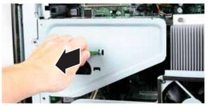
Caution Do not touch the contacts on the bottom part of the expansion card. Touching the contacts can cause electrostatic damage to the card.
